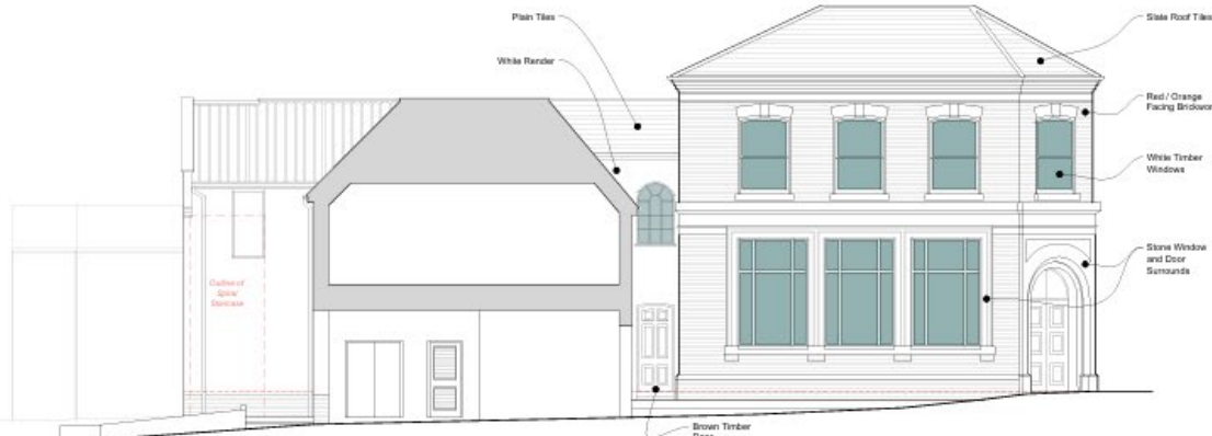
Existing East Elevation 1:100
